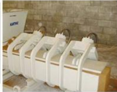
Coir Pith Block making Machine
